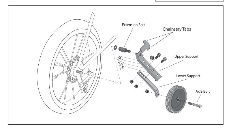
Please Note: Some hardware may not be used. This kit is intended as a universal application and contains multiple lengths and thread sizes for a variety of frame and axle styles.
