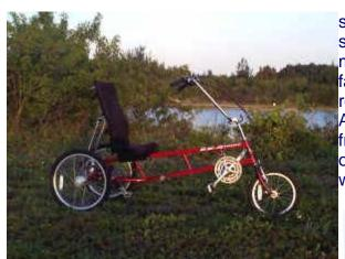
same wheelbase (56.5 inches), the same overall length (73 inches) and many of the same components. In fact, a side-by-side comparison will reveal an 80% match in specs. Although the trike's TIG welded steel frame is beefier than the EZ3's, it is ostensibly modeled after its two-wheel predecessor.
