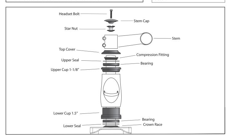
Note: Some headsets utilizes a split crown race and compression fitting - When installing, be sure that the split is NOT aligned to the centerline of the fork.
