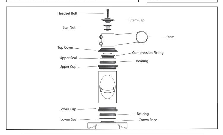
Note: This headset utilizes a split crown race and compression fitting - When installing, be sure that the split is NOT aligned to the centerline of the fork.
